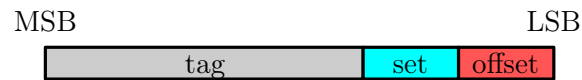
Figure 3.1: Address structure in relation to the CPU cache. The sizes of the individual parts depend on the particular architecture.
