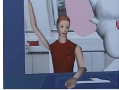
Figure 3 Remote participant, making some gesture, the gesture recognition, and the representation within the VMR, as seen through the eyes of one of the other participants.
