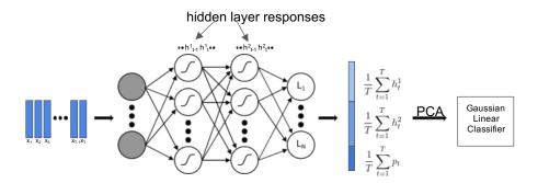
Figure 2: Proposed DNN I-vector system for LID.
