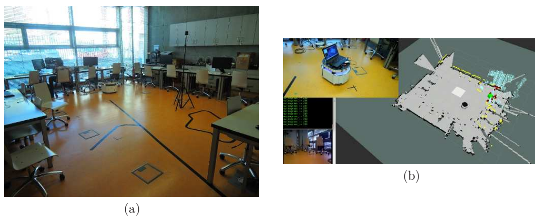
Figure 3.4: (a) Real environment. (b) RVIZ mapping together with the PatrolBot.
