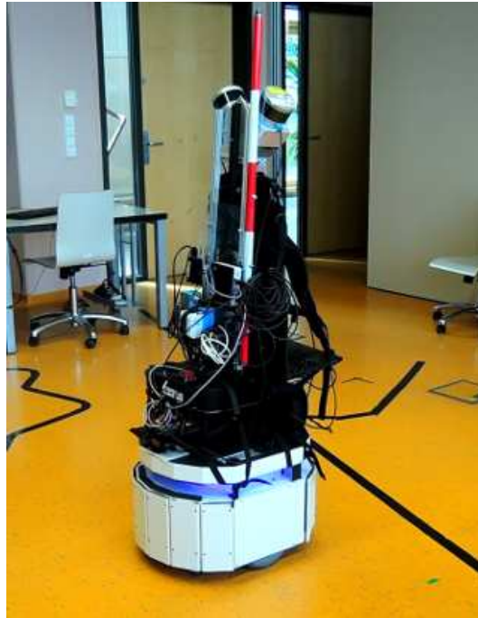
Figure 3.8: A backpack solution for 3D reconstruction based on two velodyne lidars placed on the Patrol-Bot.
