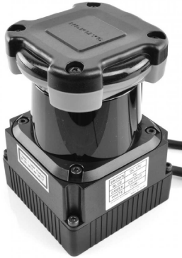
Figure 2.3: The Hokuyo UTM-30LX Scanning Laser Rangefinder.
