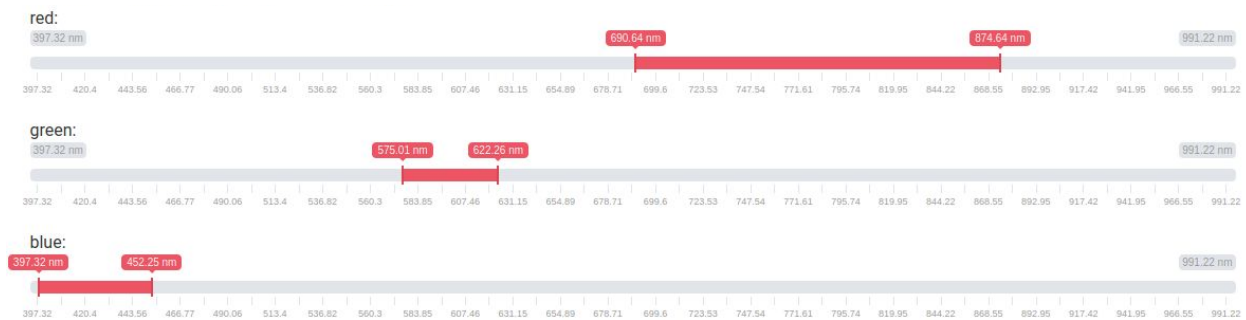
Sliders to define how a multispectral image is converted to RGB
