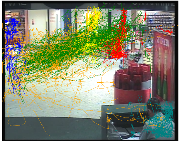
Figure 5: Examples of trajectory clustering results obtained by EM algorithm on trajectories from the first camera.
