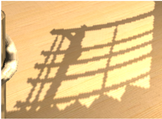
Figure 3: Shadow artefacts when using shadow map technique
