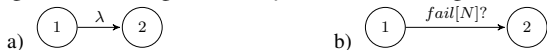
Fig. 9. Principle of converting a Markov model (a) to an STA model (b). N identifies a generator producing a fault the edge is sensitive to
