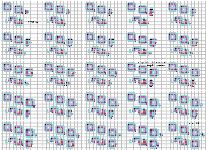
Fig. 7. Part 2 of the replication according to the transition function from Fig. 5. The sequence of steps reads from left to right and top to bottom. The development shows an autonomous growth of the loop from a non-specific structure that emerged in the last step of Fig. 6 (the bottom part of each step). It was verified that the loop is able to replicate in the same way as the initial loop during the subsequent CA development.
