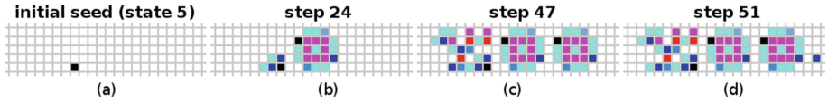
Fig. 11. A sample of the CA development from the seed according to the transition function from Fig. 10: (a) the initial seed, (b) the small loop is developed from the seed after step 24, leaving an undesirable structure on its left side, (c) the loop creates its first replica after step 47, the undesirable structure prevents from the replication on the left side, (d) the replication to the right in progress after step 51, the structure on the left no longer changes.
