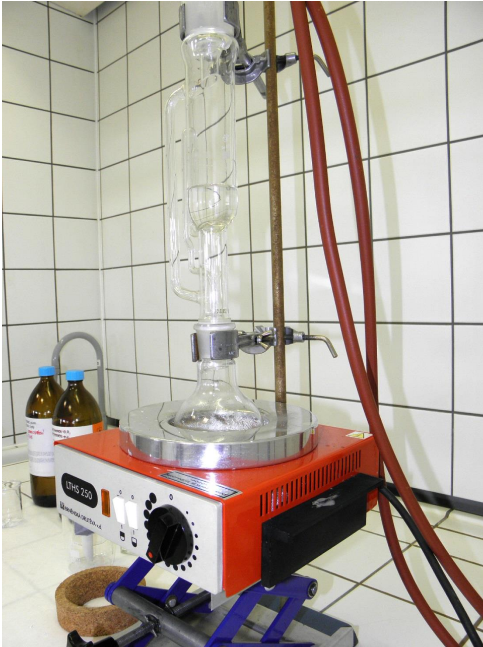
Figure 2. Boiling Nest with Boiling Acetone Bath
