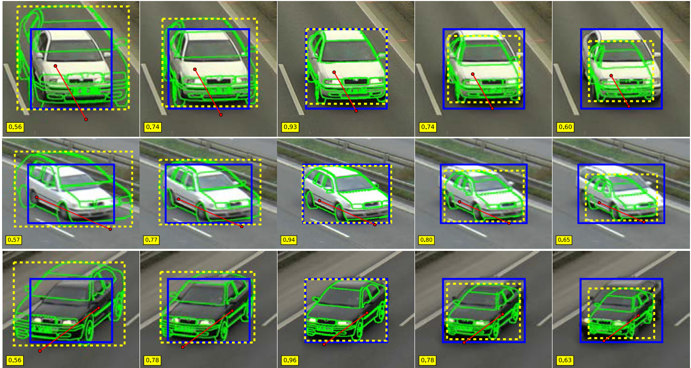
Fig. 7. Development of IoU (yellow boxes) metric for different scales (left to right), vehicle types and viewpoints (top to bottom). The left two images show larger rendered vehicles, the middle one shows the best match, and the right two images show smaller rendered vehicles. The rendered vehicle is shown only in a form of edges with the yellow rectangle bounding box of the rendered model and blue rectangle denoting the detected vehicle bounding box. (For interpretation of the references to color in this figure legend, the reader is referred to the web version of this article.)
