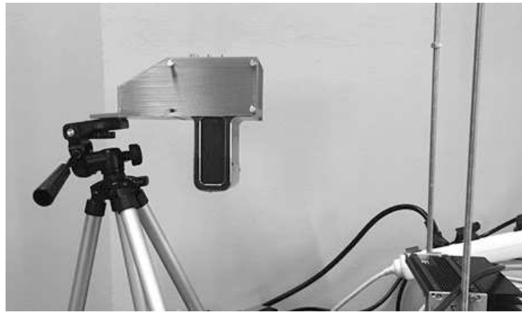
Fig. 4.25 Preview of 3DPIXA setup for 3D line scan acquisition
