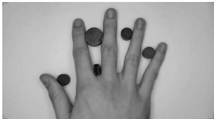
Fig. 4.1 Gathered image of a hand for 2D hand geometry extraction of features
