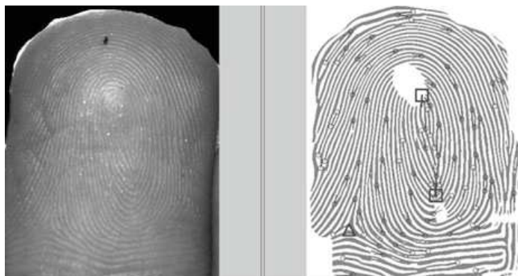
Fig. 4.21 Fingerprint image using line scanner (right), extracted fingerprint using VeriFinger SDK (right)
