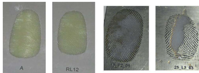
Figure 15.18 Synthetic (left) and real (right) fingerprint molds
