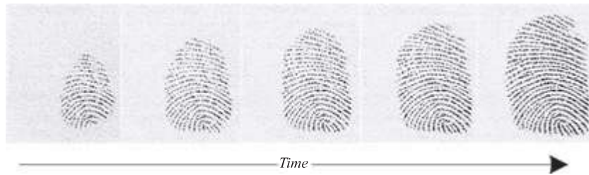
Figure 15.10 A sequence of fingerprint images describing the deformation of a real finger [11]
