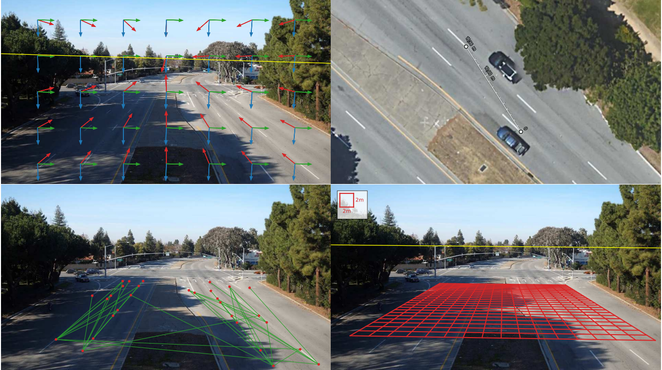
Figure 2. Top left: visualization of estimated 3 vanishing points (arrows with different color coding) and horizon (yellow line), top right: an example of used measurement on the road plane from Google Earth, bottom left: all measurements on the road plane, bottom right: final regular orthogonal grid with 2m sides.
