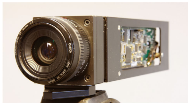
Fig. 6 Hardware prototype of HDR camera
