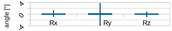
Fig. 5: Rotations (min-max) around x, y, z axis in training data sequences of KITTI dataset.
