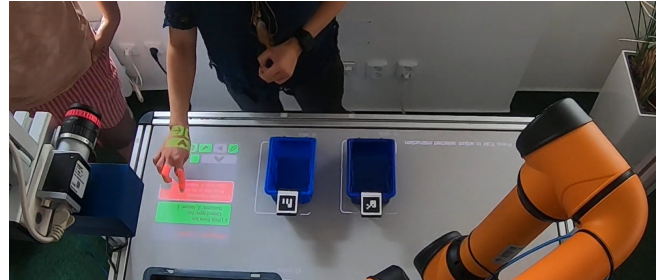
Figure 1: Participant programs a visual inspection task using the ARCOR spatial augmented reality interface.
