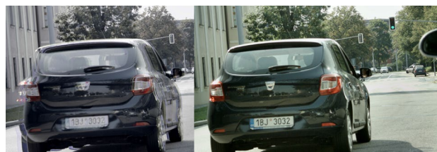
Fig. 11 A car passing by the camera—ghosted HDR (left) and result of the proposed ghost-free merging algorithm (right)
