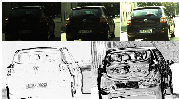
Fig. 2 Two Certainty maps (bottom) obtained from the sequence on the top. The Certainty map on the left was obtained from top left and top middle (reference) image, the Certainty map on the right was obtained from top middle (reference) and top right image
