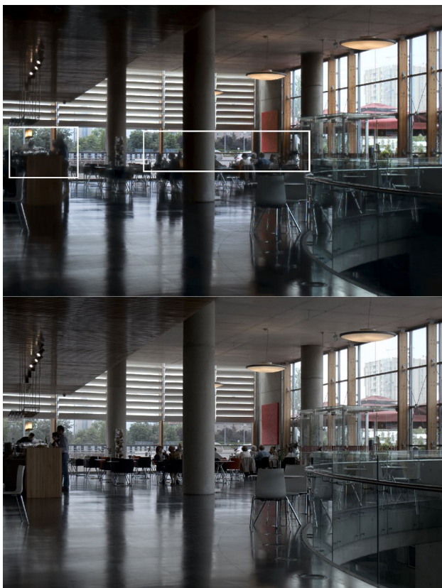
Fig. 9 Figure shows scene “Cafe” from Tursun’s [26] dataset processed with Sen [20] (top) and the proposed ghost-free algorithm (bottom). Sen [20] produce a heavily blurred image, which precludes the HDR-VDP metric [11]; moreover, the de-ghosting method fails (see marked areas, where objects are shadowed and blurred)
