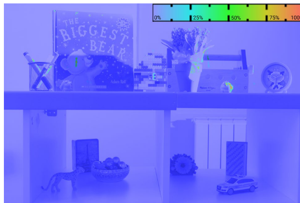
Fig. 10 Figure shows “scene 1” from Karaduzovic’s [9] dataset processed by the HDR-VDP2 [11] metric. The colour bar reflects the probability that an average observer will notice a difference between ghost-free HDR and ground truth HDR. De-ghosted HDR visual quality, according to HDR-VDP2 metric [11] is 73.24 (see Table 5)
