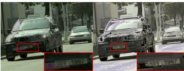
Fig. 5 Sample outputs of related deghosting algorithms [16] (left) and [12] (right) on the scene from Fig. 1. Our experiments showed that the algorithms listed should be successful only on images with convenient histogram distribution
