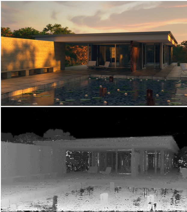
Fig. 6 Focused result using the Pavilion dataset with a correspondent focus map. The focus map contains estimated focusing value for each pixel of the final image. The map resembles depth or disparity map for the given synthetic view because the focusing values depend on the distance of the pixel from the camera.
