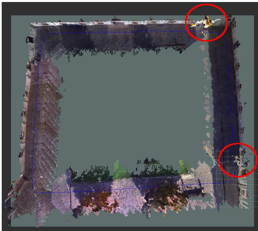
Figure 15: The blue line shows the traveled path, where multiple walls are detected.
