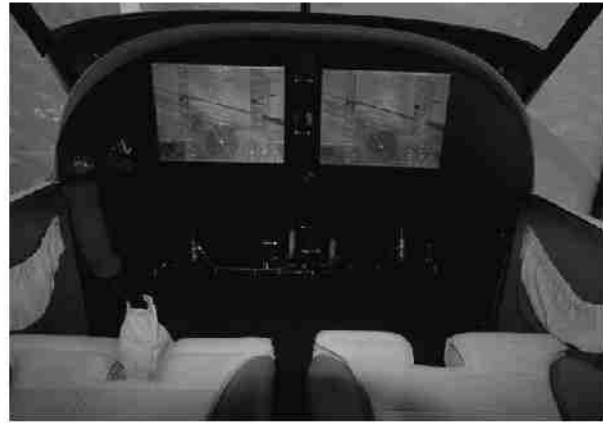
Figure 2. Glass-cockpit's displays installation.
