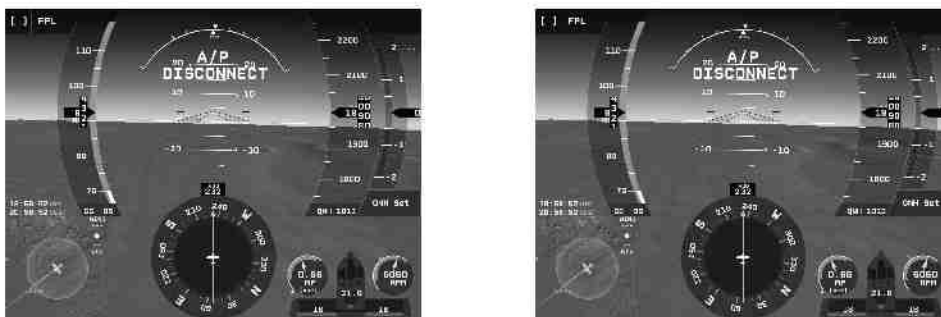
Figure 5: A/P DISCONNECT interface on PFD (left) and MFD (right)
