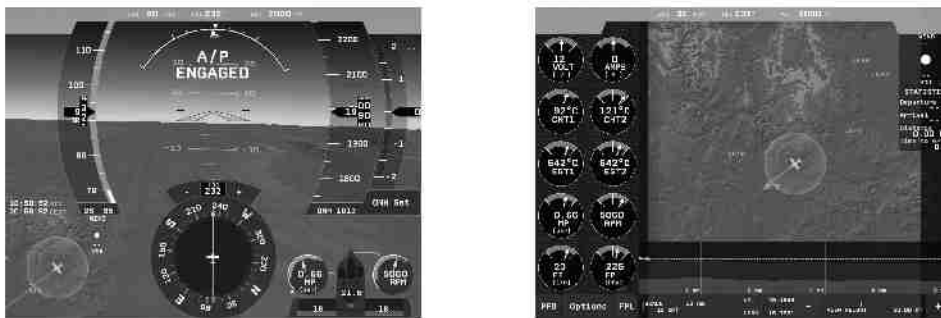
Figure 4: A/P ENGAGED interface on PFD (left) and MFD (right)
