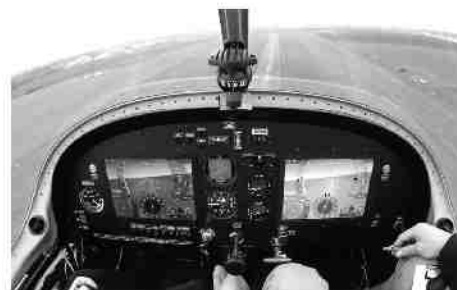
Figure 13: AFCS at final approach
