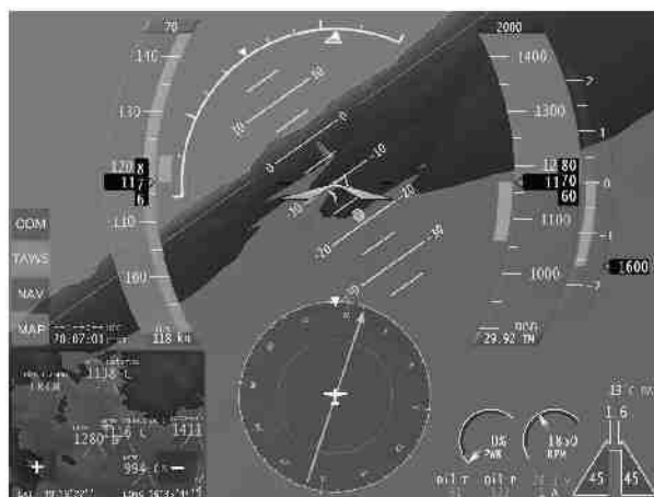
Figure 8. Potentially dangerous terrain and obstacles.
