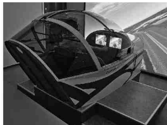
Figure 5. SimStar's Cockpit with 2 PFDs
