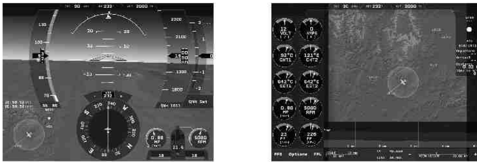
Figure 3: A/P ENABLED interface on PFD (left) and MFD (right)
