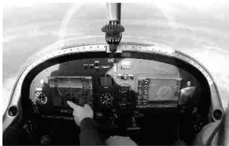
Figure 10: A/P ENGAGED – HDG
