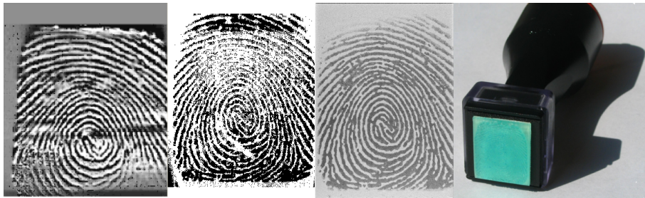
Figure 1: Left fingerprint: The stamp captured by the thermal fingerprint sensor Bergdata FCAT 100. Middle fingerprint: The stamp captured by the optical fingerprint sensor Suprema SFM3020-OP. Right fingerprint: The stamp captured by the capacitive fingerprint sensor Suprema SFM3050-TC1. Right picture: Picture of the stamp.
