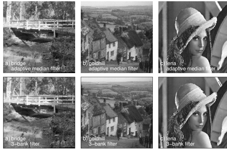
Fig. 6. Comparison of resulting images filtered using the adaptive median filter with kernel size up to 7 \times 7 (a, b, c) and 3-bank filter (d, e, f)
