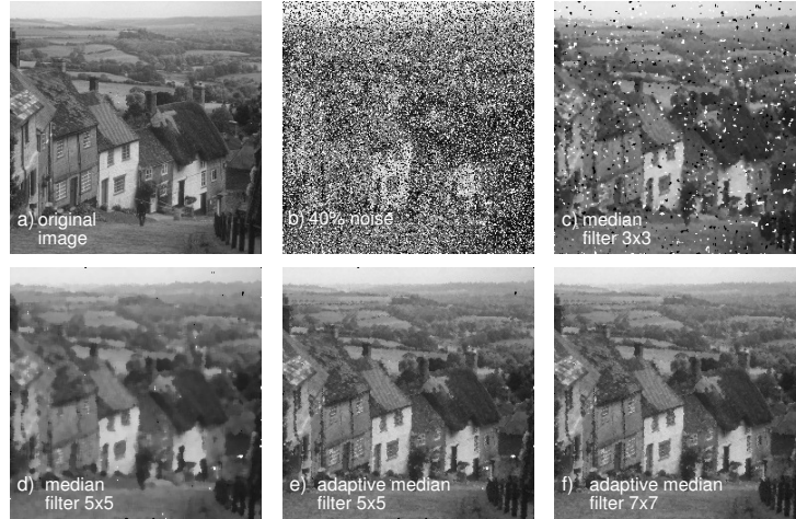
Fig. 1. Images obtained by using conventional filters. a) Original image b) Noise image corrupted by 40% Salt-and-Pepper noise, PSNR: 9.364 dB c) Filtered by median filter with the kernel size 3 \times 3 , PSNR: 18.293 dB d) Filtered by median filter with the kernel size 5 \times 5 , PSNR: 24.102 dB e) Filtered by adaptive median with the kernel size up to 5 \times 5 , PSNR: 26.906 dB f) Filtered by adaptive median with the kernel size up to 7 \times 7 , PSNR: 27.315 dB.
