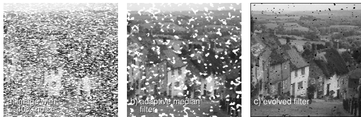
Fig. 7. a) Image corrupted by 40% impulse noise (bursts), images filtered using b) adaptive median with kernel size up to 5 \times 5 (PSNR: 11.495 dB) and c) 3-bank filter (PSNR: 22.618 dB)
