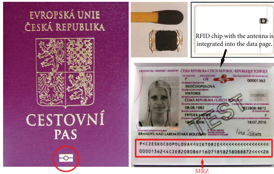
FIGURE 1: On the left: a Czech biometric passport specimen with circled international logo of electronic passports; top right: RFID chip without and with antenna; bottom right: data page with labelled MRZ (source: [1]).
