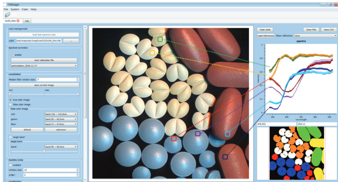
Figure 6.2: Spectral image processing pipeline of HSIImager [BM18]. The interface can be improved by implementing a feedback mechanism for which pixels would be beneficial to label.
