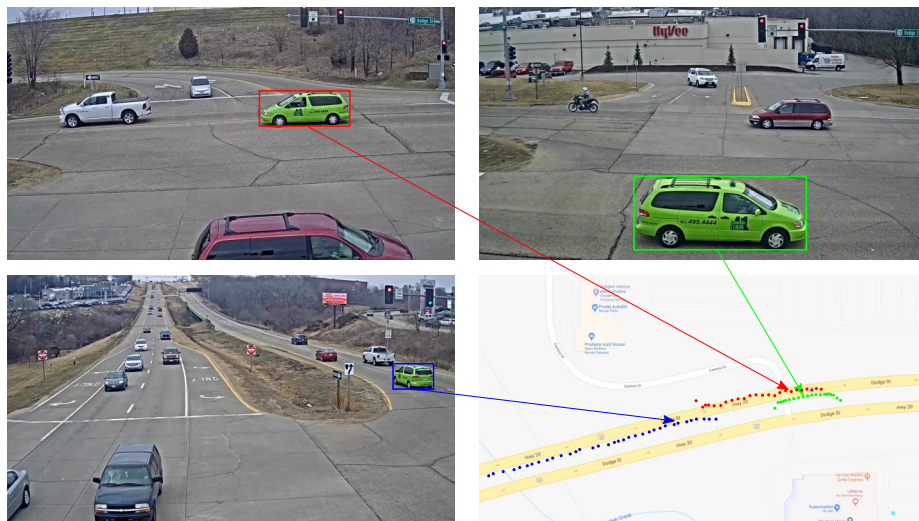
Figure 10.10: Example result of our positional matching method with a projection of trajectories’ points into a linear coordinate system. Arrows depict transformed points from image to real-world space in a specific time-step (displayed camera frame).
