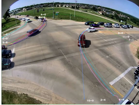
Figure 10.11: The main idea of this task — counting vehicles for every pre-defined movement of interest (travel direction).
