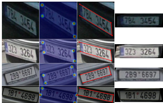
Figure 9.4: Examples of the alignment process. From left to right: input image, merged predictions, detected keypoints, aligned license plates.
