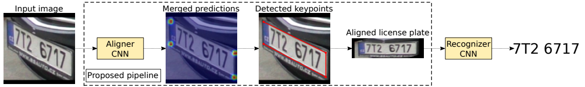
Figure 9.2: The whole license plate processing pipeline. The aligner outputs four heatmaps based on which the LP’s corner points are found and the license plate is transformed/aligned. Then, the existing state-of-the-art recognizer processes it.
