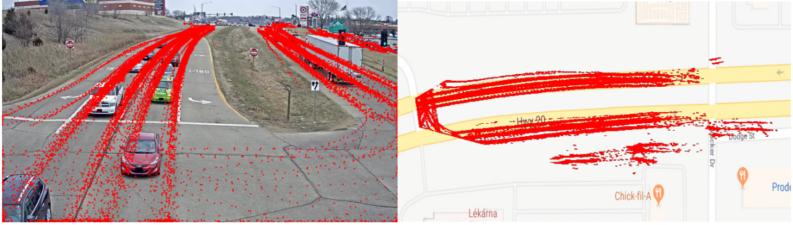
Figure 10.6: left : Detections’ bottom points used for localization of camera’s view area. right : Corresponding points transformed to the linear space (viewpoint selected as convex hull of these points).
