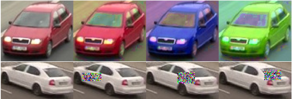
Figure 5.5: Examples of proposed data augmentation techniques. Left most image contains the original cropped image of the vehicle and other images contains augmented versions of the image ( Top – Color , Bottom – ImageDrop ).
