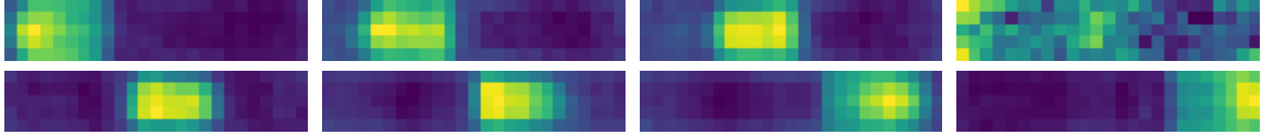
Figure 8.2: Attention of fully connected layers for different letters in the license plate. Left to right, top to bottom: 1 st to 8 th character. The 4 th letter in most cases contains the blank fill character.
