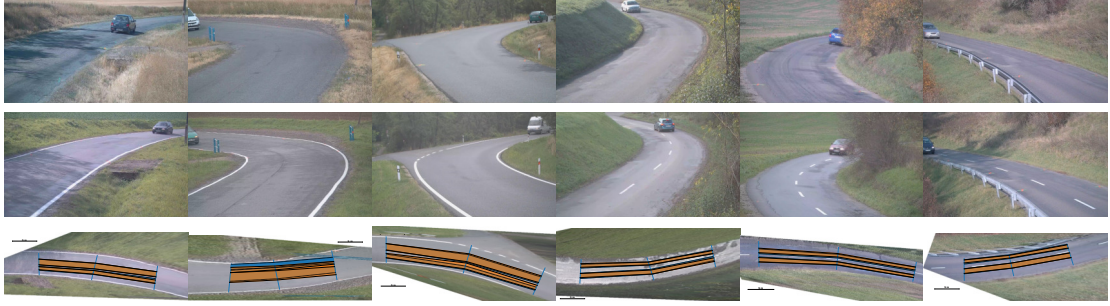
Figure 11.3: Visualization of the measured localities. top: camera view before lane markings applied, middle: view after lane markings applied, bottom: camera view projected on the ground plane computed from the calibration measurements blue color marks the envelope of trajectories prior to road marking, orange marks envelopes after road markings were drawn.
